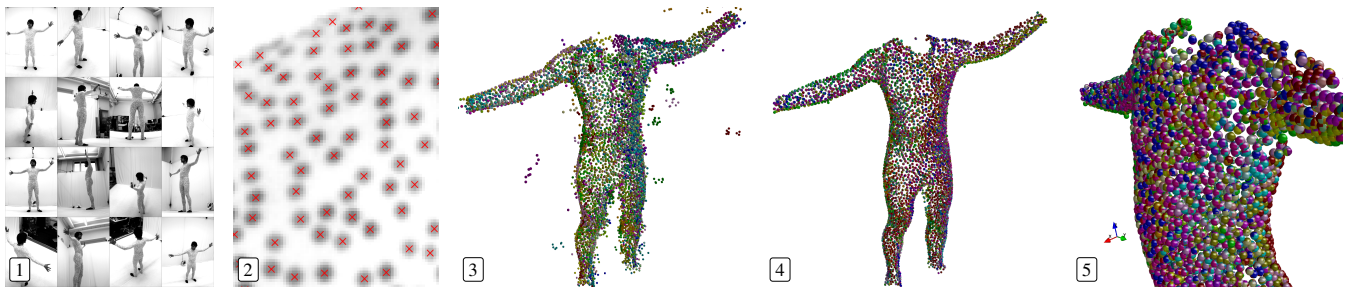
Figure 1: 3D Reconstruction with over 5,000 markers. 1) Camera images; 2) Closeup of detected markers; 3) 3D reconstruction from separate stereo matches without our multiview constraints; 4 and 5) Reconstruction by enforcing multiview constraints using our method
